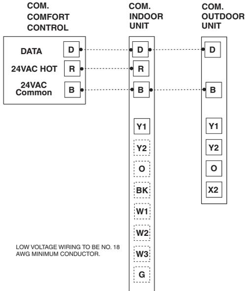
Fig. 2. Field Wiring Diagram, Communicating Indoor Unit - Communicating Outdoor Unit
