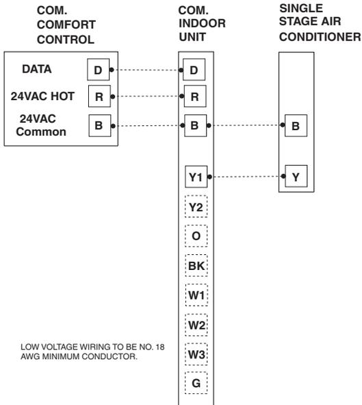
Fig. 3. Field Wiring Diagram, Communicating Indoor Unit - Single Stage Cooling Unit
