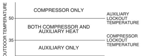
Fig. 9. Heat Pump Operation with Lockout Temperatures Set.
